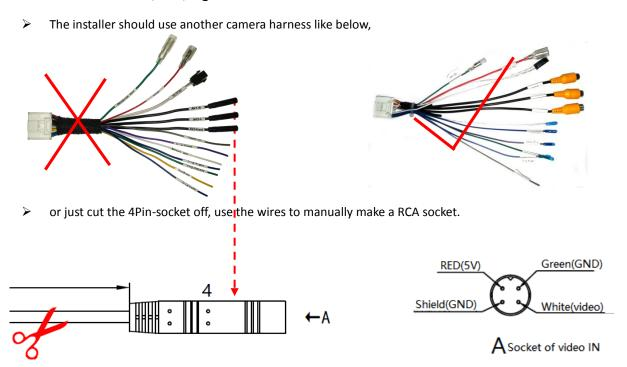
When the socket of video input is cut-off, the installer can see 4-wires inside, the definition is like left-top here. He can manually connect a RCA socket, by using the GND and Video wires.
